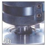
In order to avoid damage to the thread shaft, make sure that you screw in the thread shaft to a greater depth than you plan to subsequently trim off the material to.
