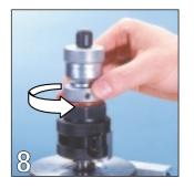
Lay the fork or ring wrench aside and turn the thrust piece to the left (counterclockwise) approx. 3-5 rotations in order to lift the steel profile up off of the work piece surface.
