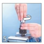
Grasp the *multicut*\* with one hand at the thrust piece and at the base part. Turn the straining ring to the right (clockwise) with the other hand until you have definitely clamped the thread shaft and affixed the *multicut*\*.
