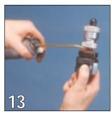
To oil or lubricate the *multicut\**, hold it on one hand and push the base part against the pressure spring, so that you can see the thread shaft. Oil or lubricate the section of the thread shaft which is visible and let the base part slide back into its original position.
