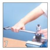
When the steel profile comes into contact with the surface of the work piece, turn the base part continuously with a suitable fork or ring wrench, thus
