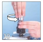
Turn the straining ring to the left (counterclockwise) until you feel the stop, thus unblocking the axial mobility of the pulling bolt.
