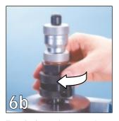
Turn the base piece occasionally in order to check if the steel profile is "free" within a range of 360°. This is recommended in case the axis of the bore hole is not squared to the surface of the work piece and an initial chip removal is expected.
