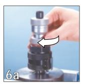
It can be useful to oil the surface of the work piece before assuming work! Turn the thrust piece to the right until the steel profile comes into contact with the surface of the work piece.
