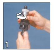
Grasp the *multicut*\*\* with one hand at the screw thread and turn the thrust piece with the other hand to the left (counterclockwise), until the cutting edge of the steel profile is far enough away from the thread shaft (normally approx. 5-7 mm).
