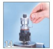
If, during use of your *multicut*\*, you should notice that when you turn the base part, the thrust piece turns along with it, adjust the pressure by means of the set screw. Use a suitable Allen key for this purpose.
