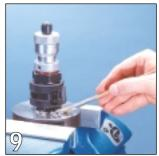
As a general principle, we recommend removing any swarf which has accumulated before you unscrew the *multicut\** from the bore hole.
