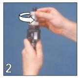
Grasp the *multicut*\* with one hand at the screw thread and turn the straining ring to the left (counterclockwise) with the other hand until you feel the stop. Do not use force!
