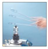
You can release the pulling bolt by lightly tapping the cap with a fork or ring wrench and the thread shaft springs back into its home position.
