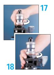
Rotate the thrust piece to the right until the measurement sensor ball contacts the sealing surface. When the measurement sensor ball contacts the sealing surface this can be seen by the deflection of the needle of the lever gauge. Rotate the thrust piece about one rotation further until the measurement sensor is pretensioned by about 0.25 mm.
