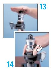
By lightly pressing with the ball of the thumb on the cap unscrew the tensioning bolts and bring the threaded shaft into the exit position.
