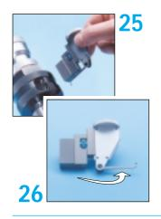
Release the two setscrews in the *multicut\**, using the Allan key take off the main adaptor with the lever gauge.
