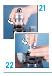
Rotate the thrust piece about 3-5 rotations to the left (anticlockwise) in order to lift the ball of the measurement sensor from the sealing surface.
