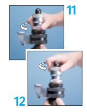
Hold the multicut\* with one hand on the screw-in thread and rotate the thrust piece with the other hand to the left (anticlockwise) until the measurement sensor is located at a sufficient distance from the threaded shaft (usually 2-3 mm, approx).
