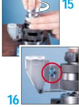
Hold the multicut\* with one hand on the thrust piece and on the main body. Rotate the tenthe main body. Rotate the tensioning ring with the other hand to the right (clockwise) until the threaded shaft is distinctly tensioned and the *multicut\** has been fixed
